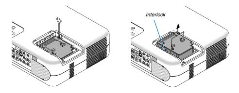
3. Insert a new lamp housing until the lamp housing is plugged into the socket.
